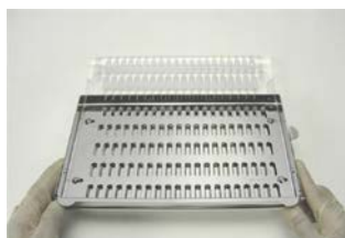
2. Slide new Orienter Tray in place.
