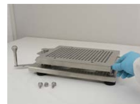
3. Unscrew 4 thumbscrews from corners of Filler Base.
