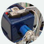
Bend Research Mill Nominal API per batch* 0.02 – 0.5 g Nominal Volume per batch* 0.5 – 5 mL
