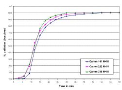
Reproducibility between manufacturing machines: three *in vitro* dissolution tests (n=6) performed with capsules from three different capsules production machines and different sizes.
