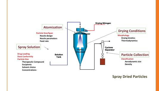
Figure 1: SD Process Used To Produce Uniform Particles for Use in Inhaled Formulations. The SD manufacturing process is tightly controlled, tunable, and scalable. The selection of the solvent, excipient type and amount, nozzle type and size, spray-solution feed rate, drying conditions and kinetics that govern particle size, drug state (amorphous or crystalline), and batch size can be altered based on the desired product profile and drug development stage.
